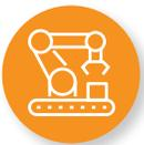
**Articulated** = robot with rotary joints
